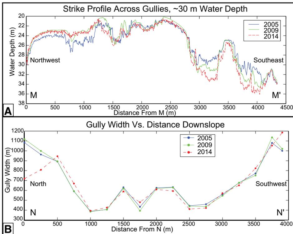
Figure 3. A: Profile M-M' across survey area showing change in gully depth between surveys. Gully depth decreases in westernmost gully, but increases in all other gullies. B: Width of Mississippi River delta front gully plotted against distance from origin along profile N-N'. Note this origin is not head of gully, but shallowest depth common to all three data sets. See Figure 2 for locations of profiles M-M' and N-N'.
