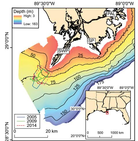
**Figure 1.** Base map showing survey area, Mississippi River Delta front, offshore Louisiana, USA. Bathymetry from Coleman et al. (1980); isobaths are at 25 m intervals. SWP—Southwest Pass; SP—South Pass; PAL—Pass A Loutre. Blue (for 2005), green (for 2009), and red (for 2014) polygons are spatial extents of bathymetric grids used in this study. Pink dashed rectangle demarcates extent of Figure 2.
