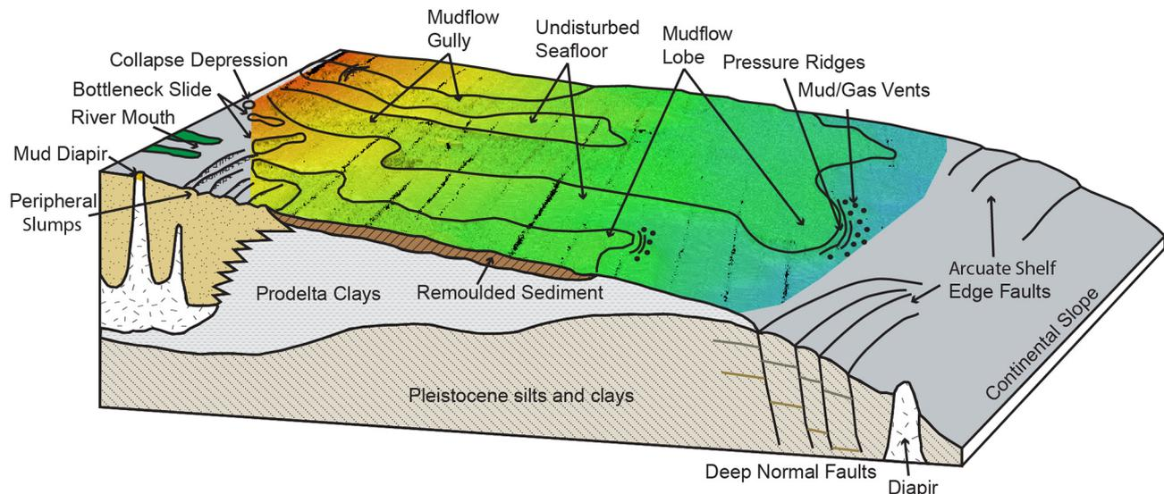
Fig. 3. Block diagram showing major instability features as defined by Coleman et al. (1980) with rainbow shaded bathymetry from Walsh et al. (2006), varying from ~15 m in red to about 60 m in blue. Cross section and deeper features not drawn to scale. (For interpretation of the references to color in this figure legend, the reader is referred to the web version of this article.)
