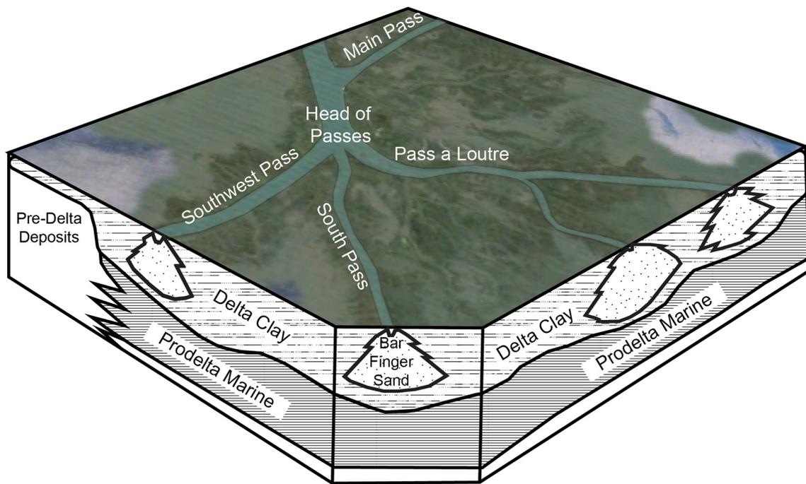
Fig. 2. Diagram depicting sub-seafloor geology of the MRDF, modified from Fisk (1961). Bar finger sands are deposited along the distributary mouths and clays are deposited away from the mouth bars. The delta sediments are built out over prodelta marine clays.
