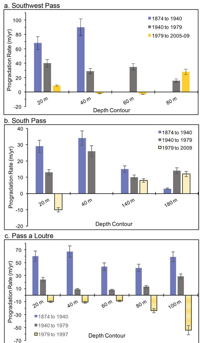
**Fig. 6.** Rates of offshore delta progradation measured at various depth contours (labeled) at a. Southwest Pass, b. South Pass, and c. Pass a Loutre. Negative progradation rates indicate retrogradation of contour lines. Error bars reflect 13% uncertainty. In A. datasets of various ages between 2005 and 2009 were used to calculate progradation rate for the most recent time interval due to lack of a recent regional dataset.
