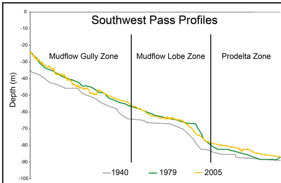
Fig. 9. Vertical profiles offshore Southwest Pass. Profile location shown in Fig. 9.
