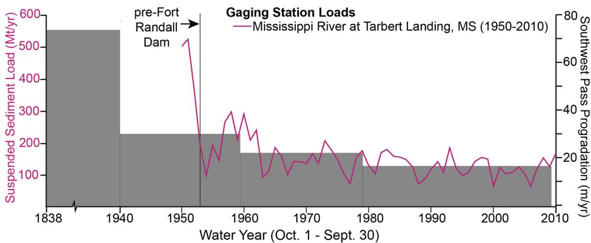
Fig. 10. Suspended sediment load of the Mississippi River as measured at Tarbert Landing (pink) compared with measured progradation rates of Southwest Pass (gray). Mt/yr = Million tons per year. (For interpretation of the references to color in this figure legend, the reader is referred to the web version of this article.)
