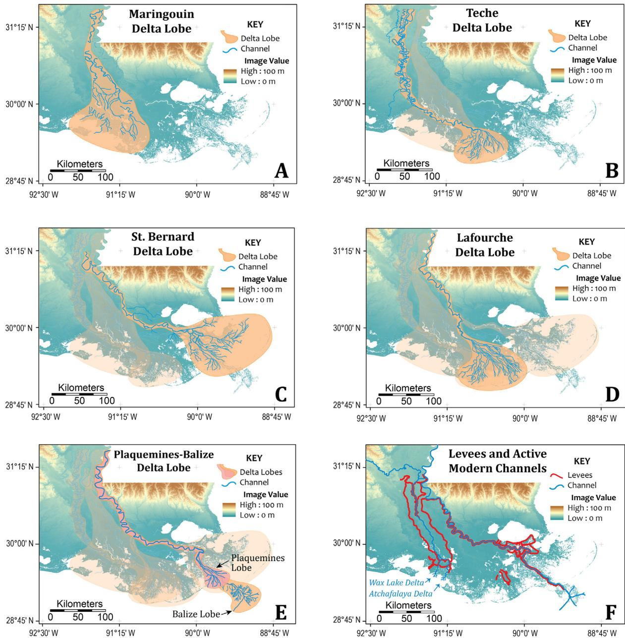
**Fig. 12.** Delta lobes and distributaries, after Fisk (1944) and Saucier (1994a). Channels and distributaries of the Maringouin complex (A) drawn by Fisk and Saucier are the least well documented. More recent cross sections identifying specific candidates for these channels are shown in Blum et al. (2007).
